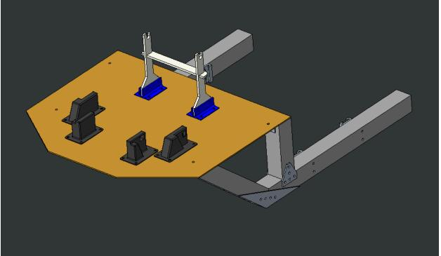
6. The final assembly should look like this and the baby chair attaches to the Tray assembly as shown below.
