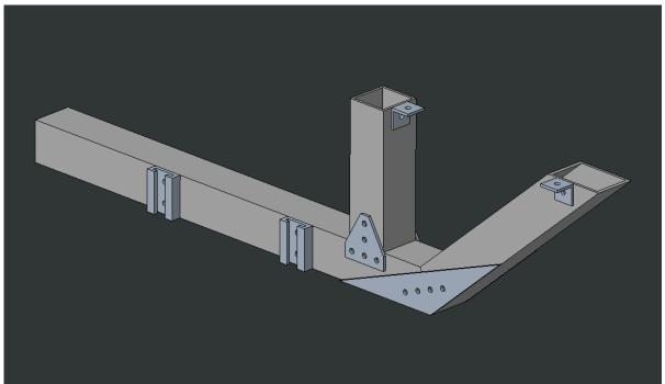
5. Repeat steps 1-4 for the remaining parts, attaching the Permobil sliding brackets and the L-bracket connected to the Angle Support beam to the opposite side of the assembly, creating a mirrored version of the first Support Assembly. The final result is shown below.
