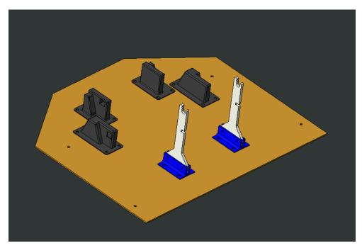
4. Use hot glue or super glue to connect the Hook Support part to the hook parts to add stability. The tray is now fully assembled.
