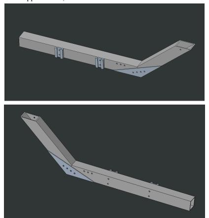
3. Use 2 T-brackets and 5 long bolt assemblies to attach the Vertical Support beam to the Horizontal Support beam as shown below.
