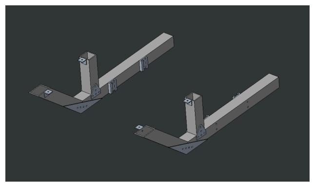
6. Slide the Permobil sliding brackets on each slide of the support over the vertical paddles connected to the rail below the seat of the M3 Permobil Corpus. Slide a pin into the topmost hole in the vertical paddles to constrain the supports in the vertical direction.
