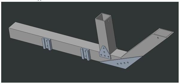
4. Use 2 L-brackets and 2 short bolt assemblies to attach one L-bracket to the top of the Vertical Support beam and another L-bracket to the top of the Angle Support bracket.
