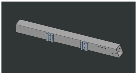
2. Use 2 Triangle Brackets and 4 long bolt assemblies to secure the Angle Support beam to the horizontal support beam, as shown below.
