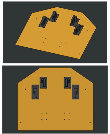
3. Use 8 short bolt assemblies to secure the hook subassemblies to the Plate as shown below.
