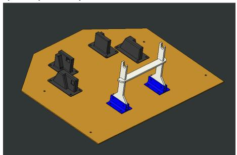
5. Use 4 short bolt Assemblies to attach the plate to the L-brackets in the Supports Assembly which is already attached to the Permobil M3 Corpus. The wheelchair is not shown in the CAD instructions below.
